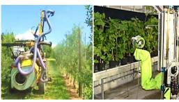
spraying robot for viticulture. The robot was successfully tested in a greenhouse environment and the attained a pesticide reduction above 80% compared to current homogenous crop treatment technique
